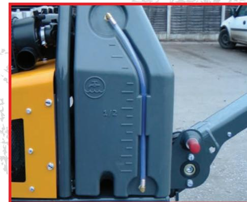
65 litre Water Tank with external gauge.
