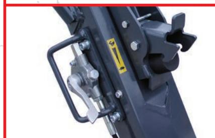
Handle mounted throttle lever, perfect for the operator
