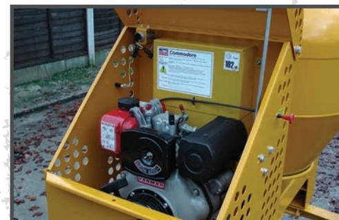
Yanmar L48 Tier V Diesel engine
