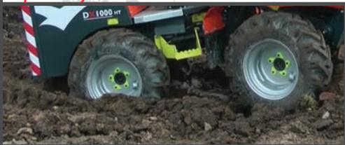
High-quality, all-terrain tyres with valve protect guard & wheel nut indicators
