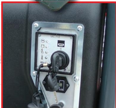
Electric, Key Ignition Start & Led Warning Lamps (Diesel Electric Model)
