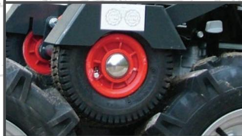
Carrier wheel disengages for easy wheel changing
