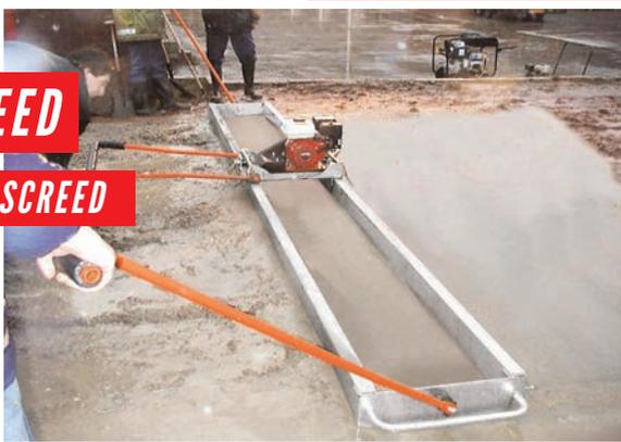
A TWIN VIBRATING BEAM SCREED FOR STRIKING OFF AND VIBRATING CONCRETE BETWEEN FORM WORK. ITS HEAVY-DUTY ROBUST CONSTRUCTION MAKES IT SUITED TO RENTAL AND DEMANDING USERS.
