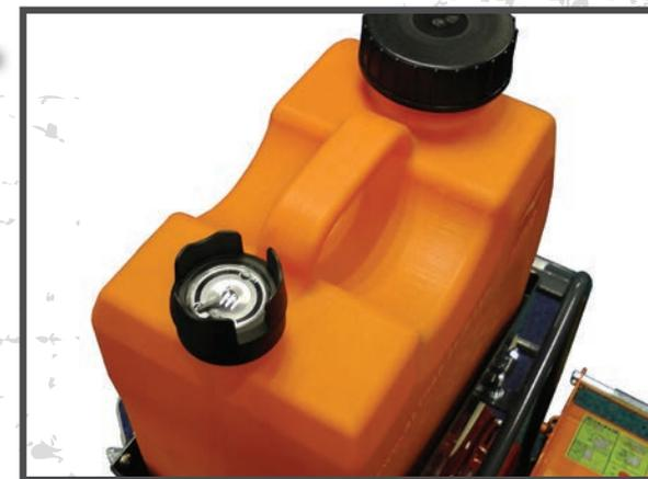
25 litre detachable water tank with built in water level gauge
