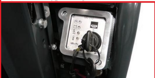
Electric, Key Ignition Start & Led Warning Lamps
