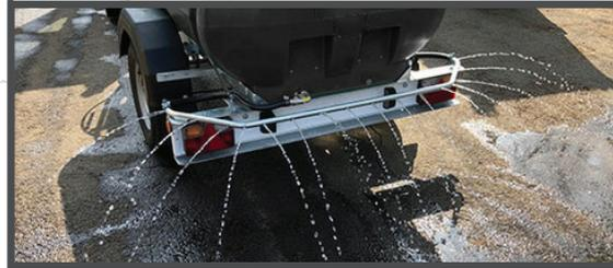
Gravity-fed spray bar option for dust suppresion
