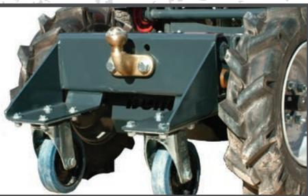
Towing-eye attachment capable of pulling 1000kg ideal for moving trailers, caravans etc.
