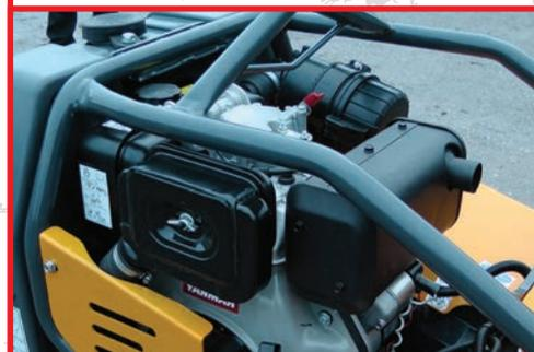
10hp Yanmar Diesel engine with back-up Recoil start
