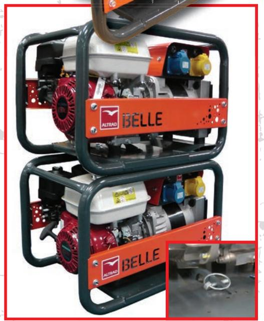
'Patent Pending' Stackable engine protection frame
